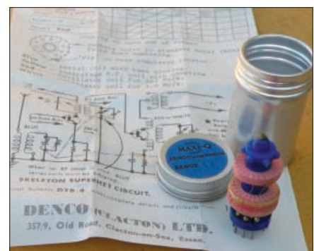
Fig. 4: A Denco B9A blue transistor range 1T (long wave) coil in front of its aluminium can and the datasheet supplied which held the coil snugly in the can during transit. The can could also be used to screen the coil, held in place by the valve socket that the coil was plugged into. Note the wave-wound coils, that are practically impossible to reproduce at home.
