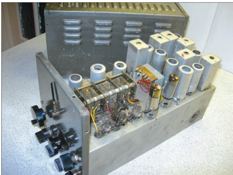
Fig. 1: The front panel and insides of the KW76 receiver, and it's clear just how compact the set was. Photo by Robin Pickering G3UWP who bought one at a rally some 20 years ago, though he's since sold it.
