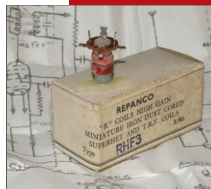
Fig. 9: A Repanco RHF3 coil perched on its box, which in turn sits on the applications sheet shipped inside the box. The applications sheet shows Repanco's address as: 116-117, Much Park Street, Coventry. Some adverts show the address as 33, Much Park Street.
