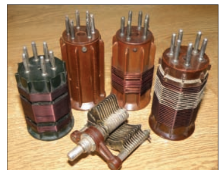
Fig. 5: Four Eddystone-like six-pin formers, plus an Eddystone 'Microdenser' tuning capacitor for company. But which ones are the real Eddystone components?
