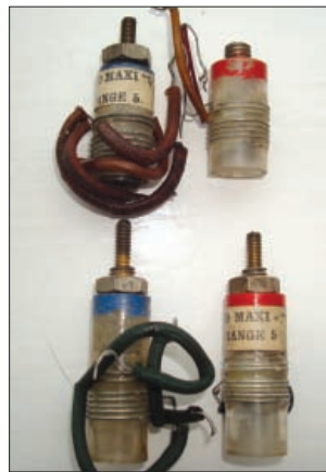
Fig. 3: Some chassis mounted Denco Maxi-Q coils (picture courtesy of Jim Jobe).
