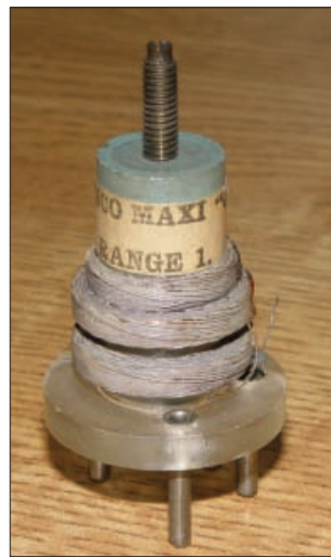
Fig. 2: A Denco octal-based valve 'dual-purpose' blue coil for range 1(long wave).
