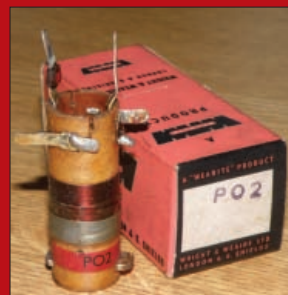
Fig. 11: A Wearite PO2 oscillator coil by its cardboard box. You can see that the PO2 part number is also printed on the coil former. The name 'Wearite' is printed 'round the back'.
